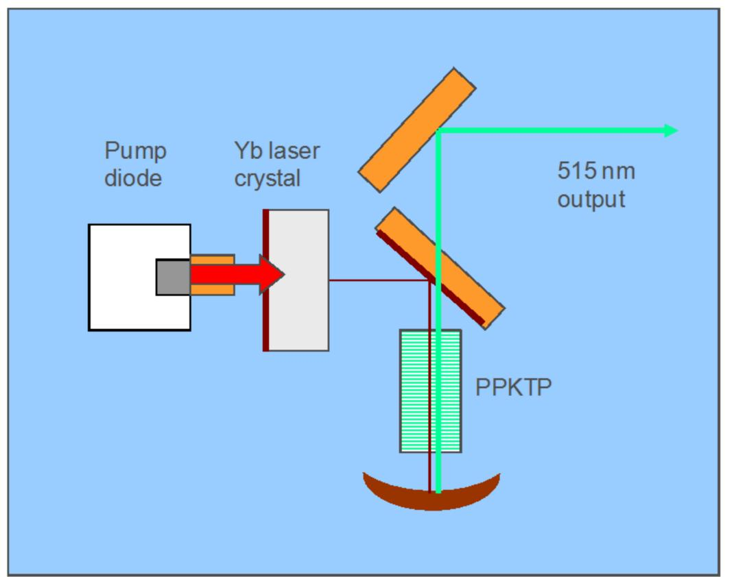
The laser cavity is enclosed in a small and robust hermetically sealed package, which provides a very high degree of resistance to varying ambient temperature and humidity conditions as well as to mechanical shocks and vibrations. Standard broad-striped edgeemitting laser diodes are used as pump sources and the laser concept is inherently power scalable.
