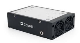
To ensure operation within given specifications, the Laser Head must be attached to a heatsink providing good thermal resistance. The value is the difference between the maximum operating laser base plate temperature (50°C) and the maximum ambient temperature at the air-heatsink interface (40°C), divided by the maximum power dissipated from the laser head (~50W). The mounting surface should be flat
