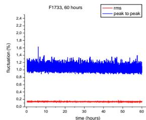
Typical noise performance of the Cobolt Mambo™ shows peak to peak noise <3% and rms noise <0.3%. This kind of single-mode DPSS laser is particularly attractive for use in demanding fluorescence analysis applications such as flow cytometry, as it provides extremely good power stability, very low intensity noise (rms<0.3%), and a nearly perfect TEM00-mode low-divergent beam ( $M^2 < 1.1$ ). These are all performance characteristics that are required for good results.
