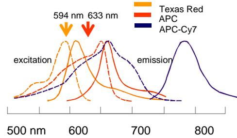
In order for researchers and instrument manufacturers to be able to take advantage of these new excitation possibilities in the orange, it is also of critical importance that suitable filters are available. Hard-coated optical filters specifically designed for a 594 nm laser are now available from Semrock, Inc (Fig.5).
