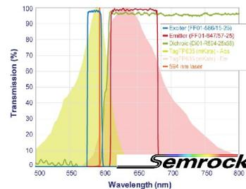
Figures 5. Hard-coated optical filters
