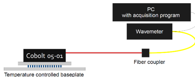
Figure 8 : Measurement setup diagram - center wavelength versus ambient temperatures
