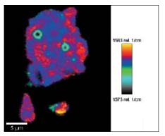
Fig. 3: Stress map obtained by peak shift analysis (lower wavenumbers: tensile stress; higher wavenumbers: compressive stress).
