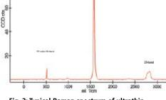
Fig. 2: Typical Raman spectrum of ultrathin Graphite.
