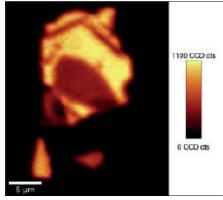
Fig. 1: Raman image of the ultrathin Graphite G-Band intensity.
