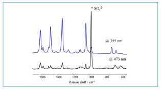
Figure 2: Raman spectra of a copper (II) complex (1 mM in water) obtained using 355 nm (Cobolt Zouk™, 10 mW) and at 473 nm (Cobolt Blues™ 50 mW). 355 nm is close to the electronic absorption of the copper (II) complex and hence the spectrum is much more intense than would be expected to be due to resonance enhancement effect.
