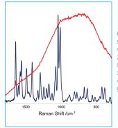
Figure 1: Near-IR dispersive Raman Spectroscopy. Comparison of the spectrum of a solid sample of an organic flurophore at 785 (red) with that obtained at 1064 nm (blue).Excitation with a Cobolt Rumba™ 1064 nm (100 mW at sample), detection 4 by 5 s exposure, Andor idus163 spectrograph with an iDus-InGaAs detector.
