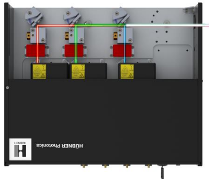
Figure 8: C-FLEX Laser Combiner with three Cobolt 05-iE lasers, 457 nm, 532 nm and 640 nm, shown with optional acousto-optic modulators in red, mounted between the laser heads and the combiner optics, which can be used for attenuation of the laser lines independently and without sacrificing stability. [8]
