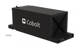
The Cobolt HS-o7 is a heatsink with fan to ensure laser operation within given specifications. The laser head must be attached to a heatsink providing low enough thermal resistance to its environment. The HS-o7 is powered by the PSU that comes with the lasers via an adaptor cable used between the laser and the fan.
